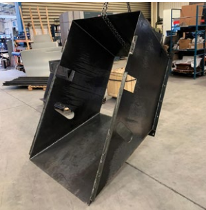
Ash hopper during fabrication as a direct replacement to an existing unit.
