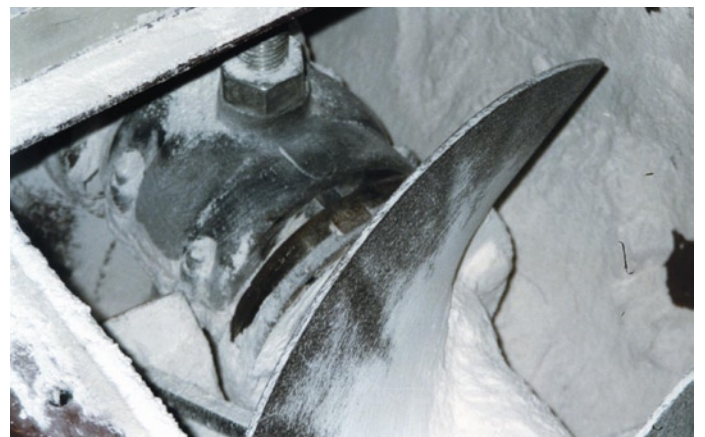
Standard hanger unit on a screw conveyor
