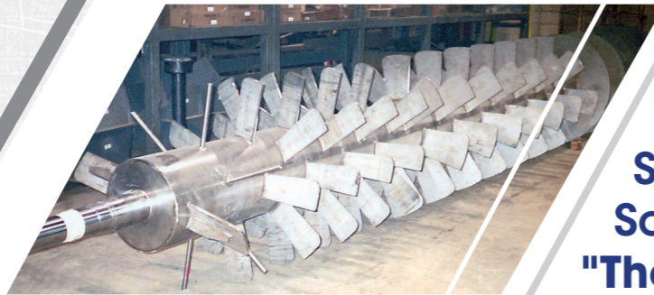
30' (9.525 cm) long, 48" (121.92cm) diameter 316 stainless steel paddle type screw made by Martin.
