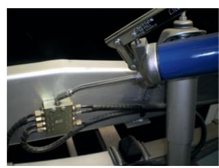
**Helps Maintain Long Term Machine Performance** – the positive displacement of grease through the progressive system ensures each grease point receives the correct quantity of grease.
