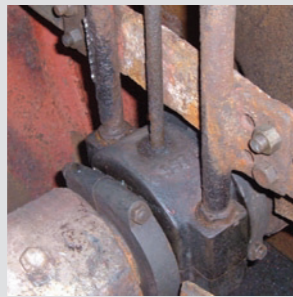
SCREW CONVEYOR EQUIPPED WITH A TROUBLESOME PLAIN BEARING BEFORE CONVERSION
