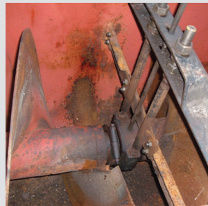
SCREW CONVEYOR EQUIPPED WITH A TROUBLESOME PLAIN BEARING BEFORE CONVERSION
