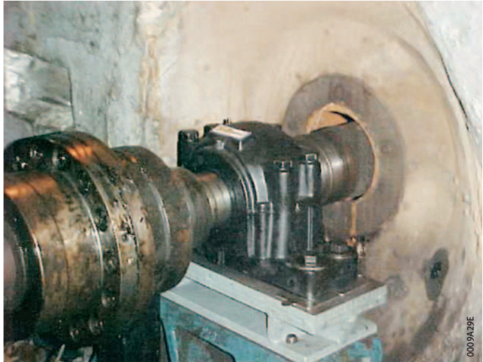
Figure 6 Bearing arrangements in fans and ventilators
