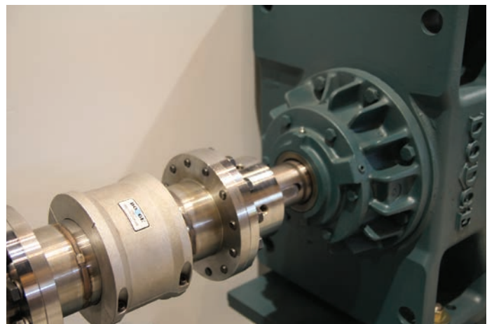
Figure 1 Dodge Grid-Lign spacer coupling mounted between a Baldor•Reliance motor and a Dodge MagnaGear reducer
