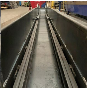
A new precipitator dust conveyor during manufacture and prior to entering the paint shop.
