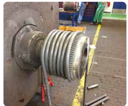
Heating a coupling for dismounting
