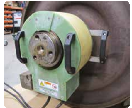
Heating bearing rings for dismounting
